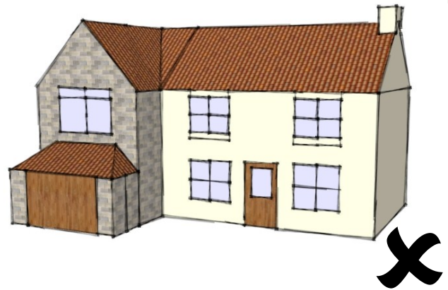
Inappropriate extension coming forward of the property and dominating the host property
